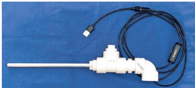
Figure 1. Arthroscope simulator.
