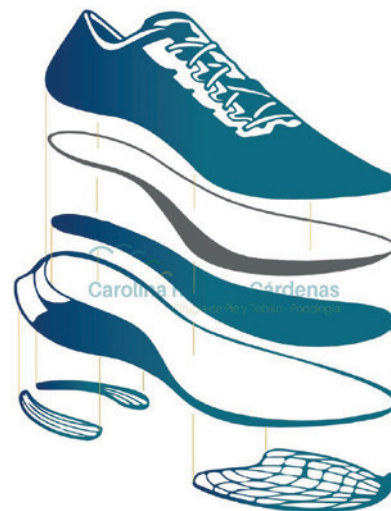
Figure 5. The midsole is formed by layers of foam that provide cushion; in between, some shoes provide more rigid materials such as carbon plates or TPU that provide stiffness.
