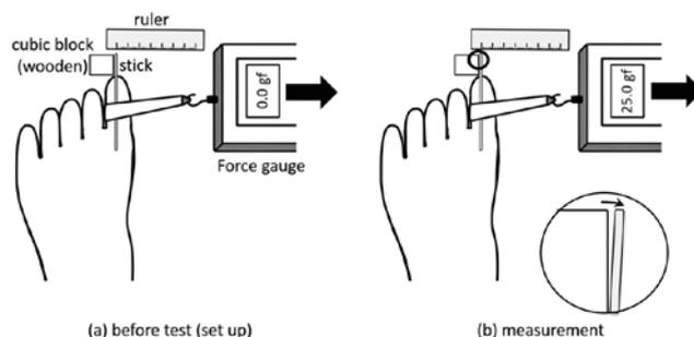
Figure 3. Initial movement value test is shown schematically.
