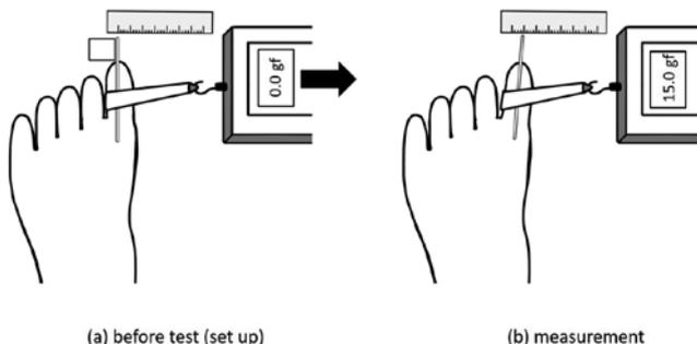
Figure 4. The traction value test is shown schematically.
