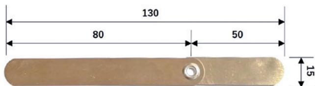
Figure 1. Super-elastic alloy brace with a hinge joint.
